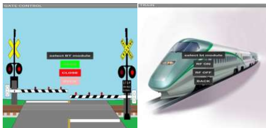
Figure: 6 Mobile application – manual and automatic gate operation screen
