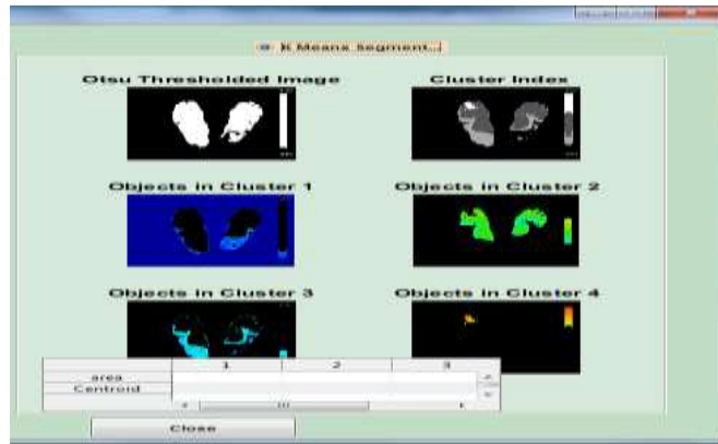
Fig-12: Segmentation with K-means clustering for different objects with cluster index
