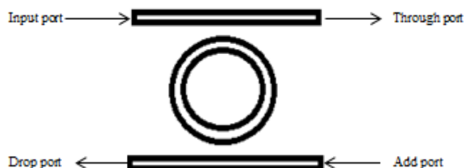
Fig-1: Schematic of a Ring Resonator.
