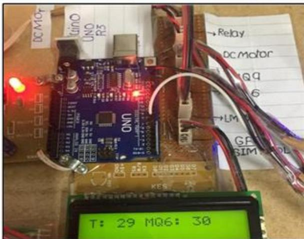
Figure 8: Display showing the value from LM-35 and MQ6 sensors
