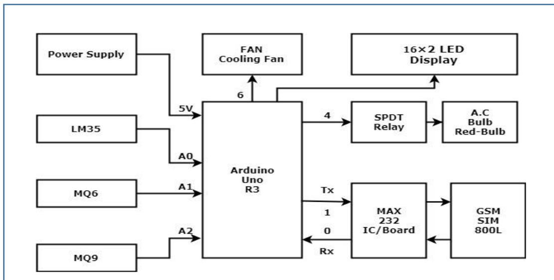
Figure 1: Block Diagram of proposed Systems.
