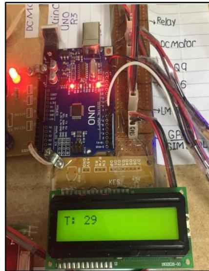
Figure 7: LCD Display shows the temperature
