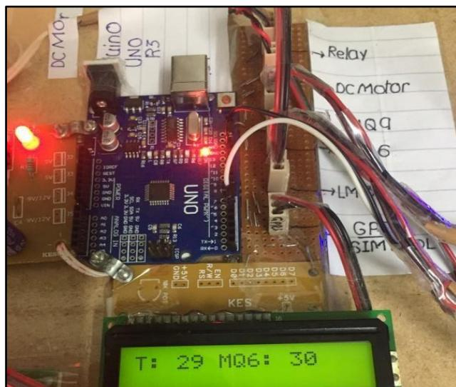
**Figure 8:** Display showing the value from LM-35 and MQ6 sensors
