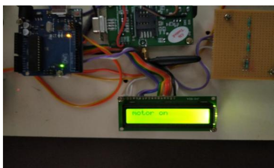
Figure 3: the LCD display that shows motor ON
