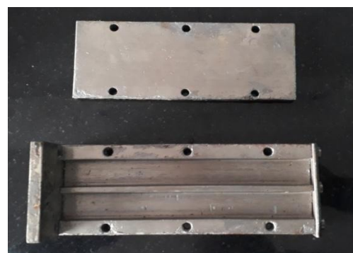
Figure 2: Composite Specimen For Mechanical Testing Filled With SiC & h-BN
