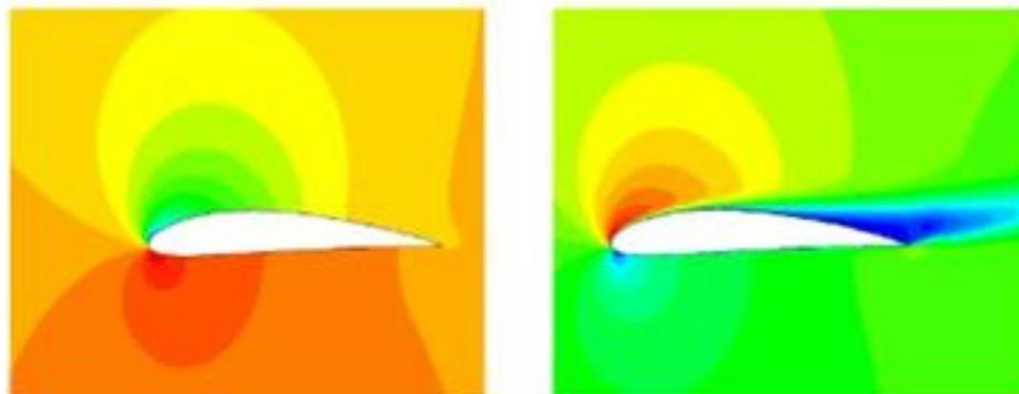
Fig-5: Stationary pressure also velocity contour at 120° position of attack
