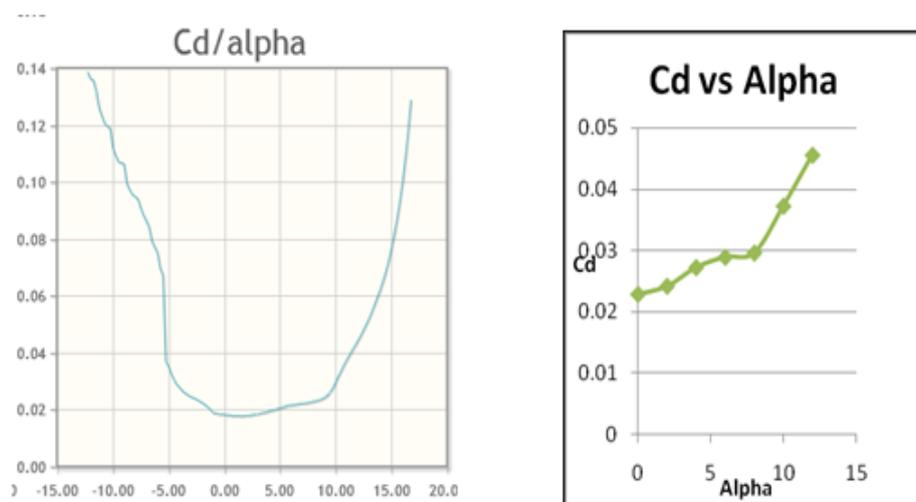
Fig.-10: Evaluation of CD at 0° to 12° position of attack
