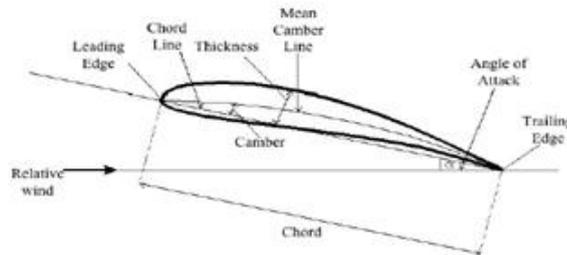
**Fig.2:** Fundamental geometry of the airfoil
