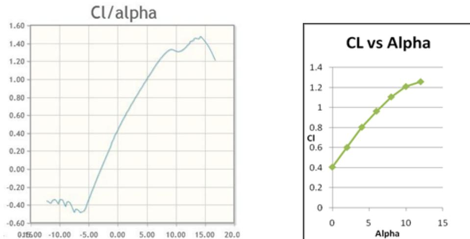
**Fig.-9:** Evaluation of  $C_L$  at 0° to 12° position of attack
