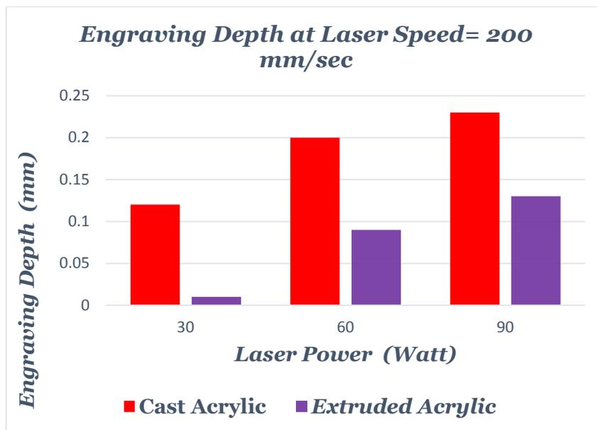
Fig.7 Laser engraving depth at Cutting Speed= 200 mm/sec
