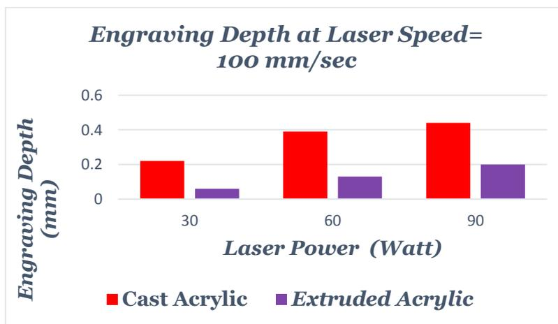
Fig.5 Laser engraving depth at Cutting Speed= 100 mm/sec
