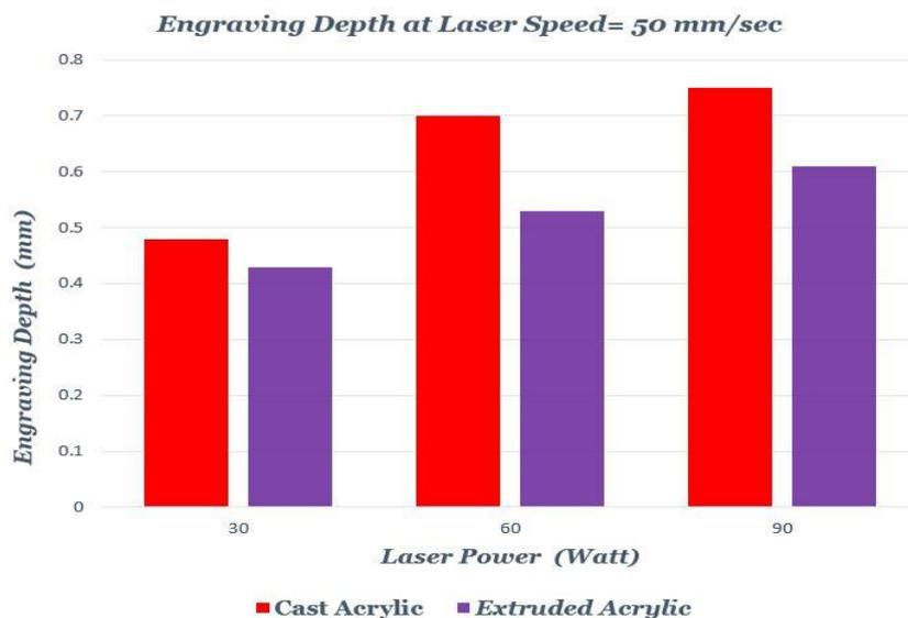
Fig.4 Laser engraving depth at Cutting Speed= 50 mm/sec
