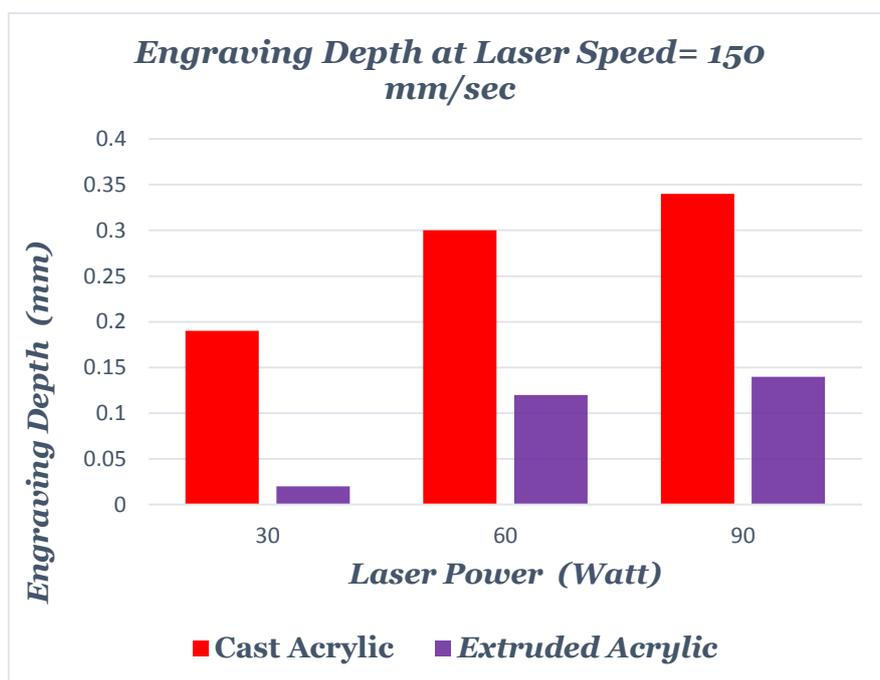
Fig.6 Laser engraving depth at Cutting Speed= 150 mm/sec
