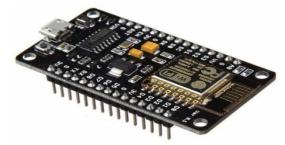
The ESP8266 has **17 GPIO pins (0-16)**, however, you can only use 11 of them, because 6 pins (GPIO 6 - 11) are used to connect the flash memory chip. This is the small 8-legged chip right next to the ESP8266.
