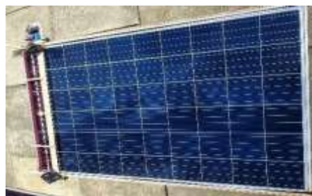
Figure 2: Complete setup of the solar panel cleaning system.
