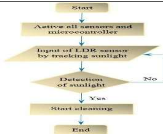
Figure 5: Flow chart of the program used for solar panel
